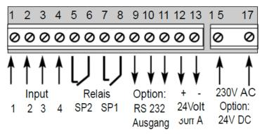
Fig. 2: Terminal assignment of the terminals
