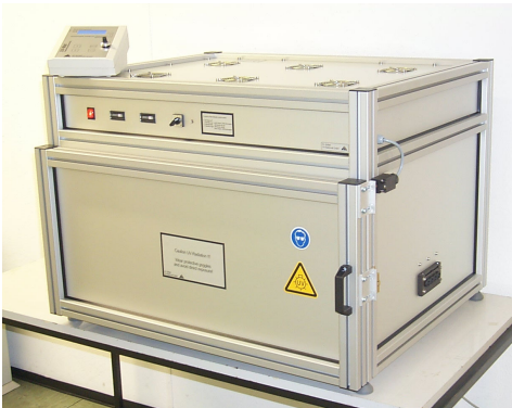
Fig. 1: UV/VIS irradiation chamber BS-04 with dose control UV-MAT
