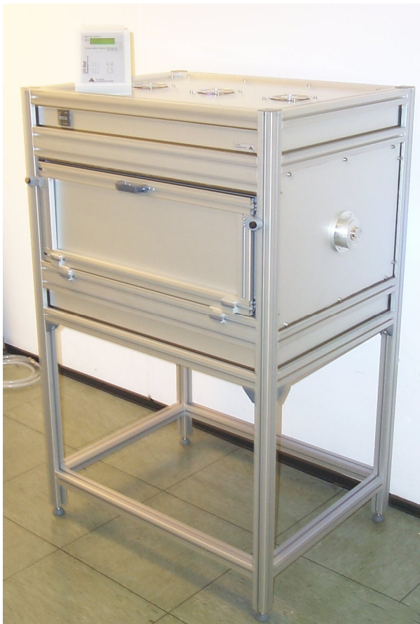
Fig. 1: UV/VIS irradiation chamber BS-05 with dose control UV-MAT
