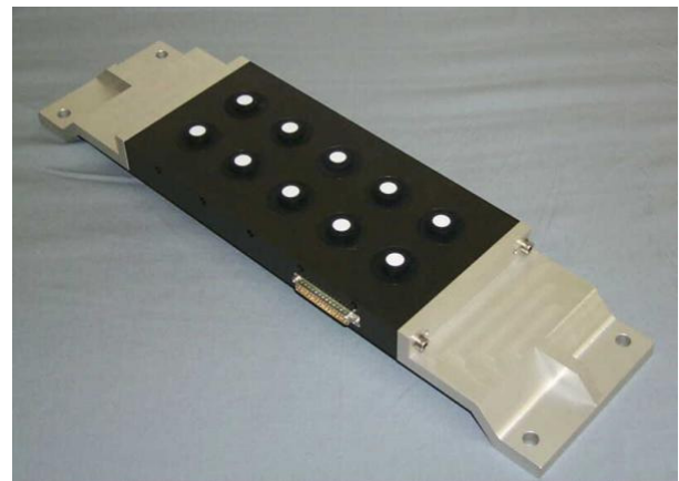
Fig. 4: Sensor plate with 10 UV-sensors for 10 light guides
