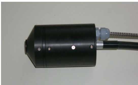
Fig. 2: Reflector head for colour measurements
