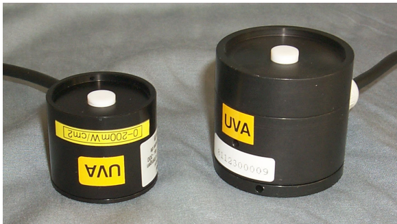
Fig. 1: Radiometer UV sensor (Standard version on the left, IP65 on the right)
