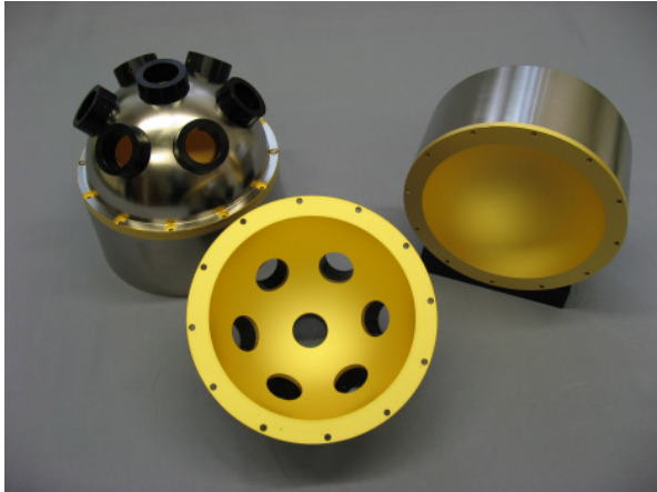
Fig. 3: 175 mm integrating spheres with 20 µm diffuse gold plating for the infrared spectral range
